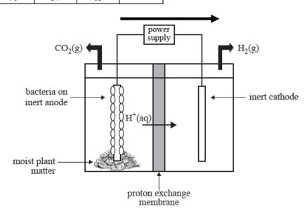
Students were expected to show that the electrons move from left to right (from the site of oxidation to the site of reduction) and in the external circuit. The most common errors showed electrons moving through the proton exchange membrane or in the wrong direction.
