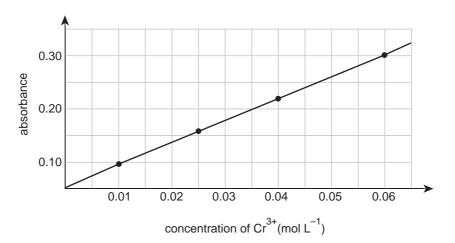
A solution was prepared by dissolving 15.0 g of steel containing 6.02% Cr by mass in acid, and making the solution up to a total volume of 300.0 mL.
