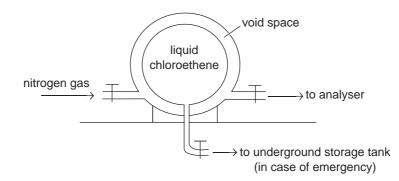
Nitrogen gas is flushed through the space and analysed to detect any leaks of chloroethene.
