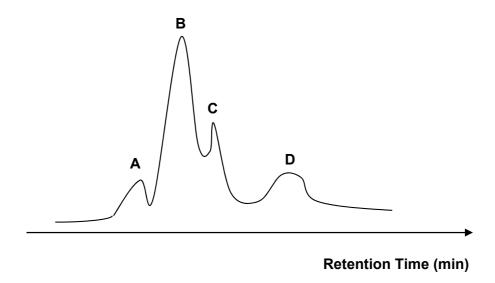
A sample containing a mixture of ethanol, ethanoic acid, propanol and propanoic acid was injected into the top of the column and vapourised.
