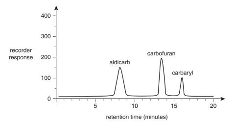
A sample of the town water was analysed by HPLC under identical conditions, resulting in the chromatogram shown below.
