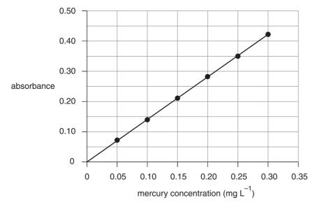
The absorbance of one solution from a soil sample was 0.58. The following suggestions were made to overcome the inadequacy of the calibration graph.
