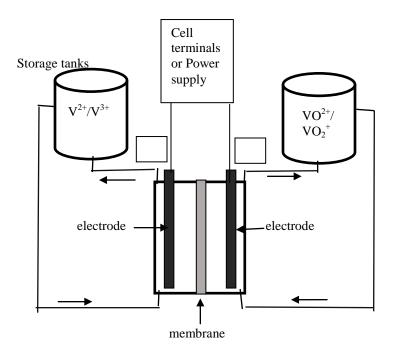
The left hand storage tank contains  $V^{3+}$  ions and  $V^{2+}$  ions. The right hand tank contains  $VO_2^+$  ions and  $VO_2^{2+}$  ions.
