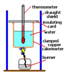
Ethanol is placed in the burner and 150g of water is poured into the copper "calorimeter". The wick of the burner is lit and after 2.0 minutes, the mass of fuel has decreased by 0.873g and the temperature of the water has increased from 18.0°C to 41.5°C.
