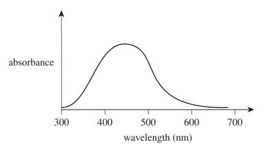
UV-visible spectroscopy is to be used to determine the concentration of the colouring in the wastewater.
