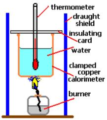
When propan-1-ol is burnt, the mass of the spirit burner decreases by 0.560g and the temperature of the 100 mL of water in the can increases by 25.3 °C.
