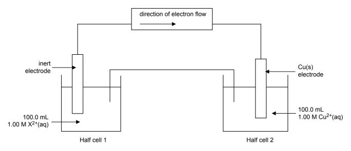
After discharging 2654 C of electricity, the concentration of the  $X^{2+}(aq)$  in solution in half cell 1 was found to be 0.725 M. The volume of the solutions in the two half cells had not changed.
