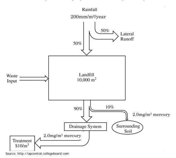
a. Calculate the volume, in m<sup>3</sup>, of the water infiltrated through the landfill per year.
