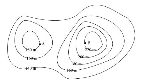
Two hills are shown on the contour map above. The horizontal distance between point A and point B is 70 metres. A bird flies in a straight line from point A to point B.
