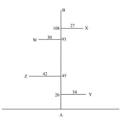
A field sketch of a traverse survey is shown in the diagram above. The vertical base line AB has 4 horizontal lines branching off it and these lead to points of interest which are represented by W, X, Y and Z. The distance, in metres, from each of these points of interest, horizontally back to the base line is indicated in the diagram as is the distance from A to each point where one of the horizontal lines branches off.
