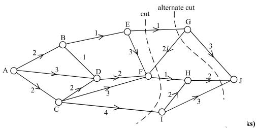
The first cut has a capacity of 1+1+4=6. The alternate cut has a capacity of 1+2+3=6.
