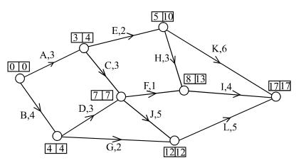
On the network above near each node are two numbers. The first is the earliest start time and the second is the latest start time.
