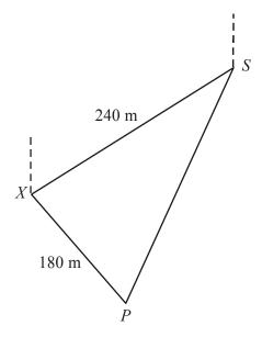
In the diagram above, the building under construction is located at point X. In relation to point X, the bearing of the train station, S, is  $065^{\circ}$  and a direct distance of 240m away. Also, a post office P, is on a bearing of  $215^{\circ}$  from the station and its direct distance from X is 180m.
