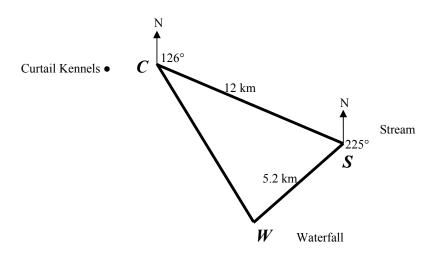
a.  $\angle S = (360 - 225) - (180 - 126) = 81^{\circ}$   $CW = \sqrt{12^2 + 5.2^2 - 2 \times 12 \times 5.2 \cos 81} = 12.31 \text{ km}$ The distance is 12.3 km
