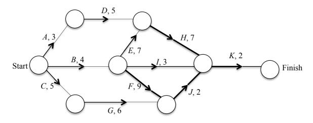
The graph above shows activities that must be completed to finish a project and the completion time in days for each activity.
