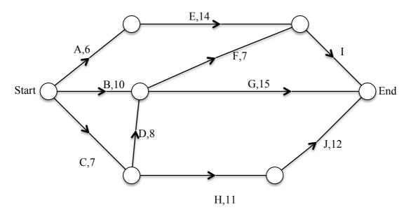
The above network shows the activities that must be completed before the cable for the Internet is ready for use.
