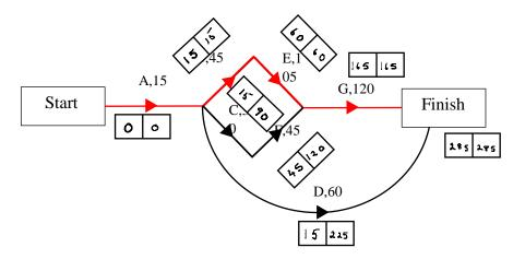
The critical path is  $A \rightarrow B \rightarrow E \rightarrow G$  with a completion time of 285 hours.
