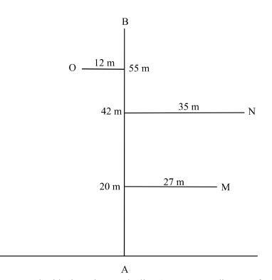
The measurements beside the points on the line AB represent distances from point A which is on the base line.
