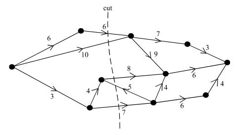
For the graph shown above, the capacity of the cut indicated is
