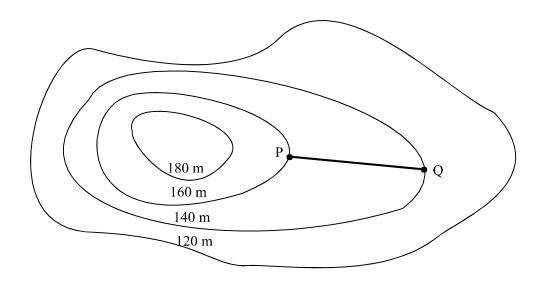
The distance between the points P and Q on the contour map is 10 mm. The average slope of the line joining points P and Q is
