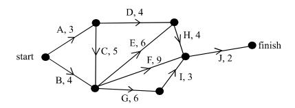
For the network shown above, the time taken, in weeks, for each of the respective tasks A, B, C,..., are indicated on each of the arcs. The earliest start time, in weeks, after the project has started for activity J is
