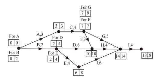
The left hand number in the boxes near the vertices gives the earliest start time for the activity. The right hand number gives the latest start time for the activity. The critical path is *ACFHJ* since the earliest and latest start times are equal for the activities on that path. The length of the path is therefore 3+4+3+4+4=18. The answer is C.
