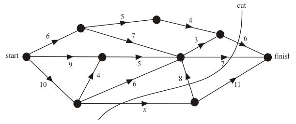
There are no cuts possible with a capacity of 18 that don't include side *x*.
