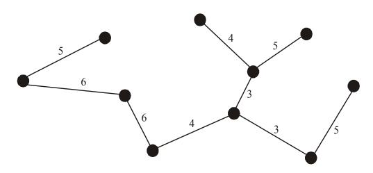
The minimum spanning tree is shown above. It started at one of the edges with a length of 3 and extended via the branches with the shortest length until all vertices belonged to it. The total length is 3+3+4+5+4+5+6+6+5=41The answer is C.
