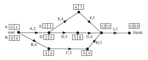
**a.** Using our earliest start time and latest start time boxes we see that the shortest time in which the upgrade can be completed is 15 days.
