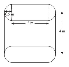
The height of the water tank is 4m and the length is 4m. The radius of each semi-circular cross-section is 0.5m and the length of the rectangular cross-section is 3m as indicated in the diagram.
