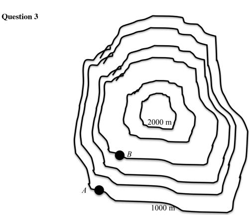
The contour map above has contour intervals of 200 m. The horizontal distance between A and B is 1 km. The angle of elevation from point A to point B is closest to
