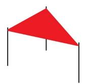
To build the shade sail, posts must be installed to hook the sail to, as shown above.
