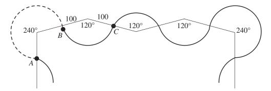
Each arc section has radius 100 metres. The subtended angle is  $120^{\circ}$ , except at the corners where the angle is  $240^{\circ}$ .
