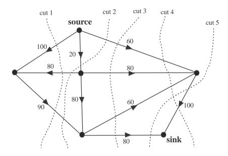
Five cuts are drawn on the diagram and one of them is the minimum cut for this network. The maximum flow of liquid, in litres per hour, that can flow from the source to the sink is
