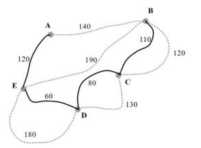
The minimum length of bunting used to connect the pergolas would form a minimal spanning tree that can be determined using Prim's algorithm.
