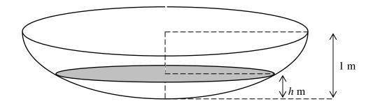
The diagram above shows a pond with water filled to a depth of h m. The shaded part is the water surface and has an area  $A = 2\pi \left[1 - (1 - h)^2\right]$  m<sup>2</sup>. The volume of water is  $V = 2\pi \left[\frac{2}{3} - (1 - h) + \frac{(1 - h)^3}{3}\right]$  m<sup>3</sup>.
