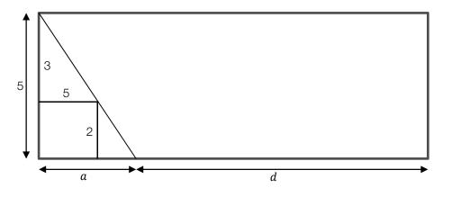
Using similar triangles,  $\frac{a}{5} = \frac{5}{3}$  [2 marks for diagram and explanation]
