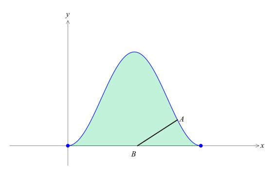
The curve has the equation  $y = 2 - 2\cos\left(\frac{\pi x}{3}\right)$ ,  $0 \le x \le 6$ . All measurements are in metres.
