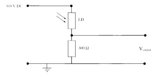
What is the output voltage of the circuit if the LDR is illuminated by light with an intensity of 20 lux?
