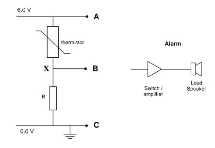
The voltage must drop below 5.0 volts for the alarm to work correctly.
