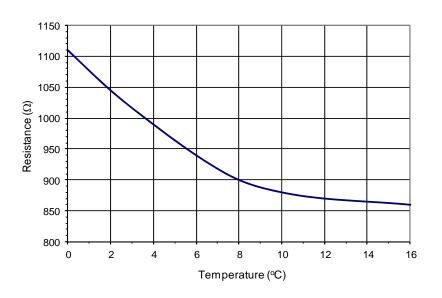
Thermistor Resistance vs Temperature
