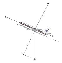
As shown in the diagram above, this means that some of the weight force (that is, the component parallel to the plane's flight path) must be compensated for by an increase in thrust.
