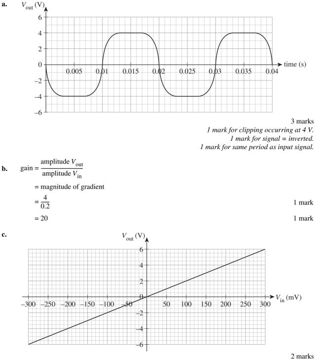
*1 mark for positive gradient of value 20. 1 mark for amplification region allowing –250 to 250 mV as minimum domain.*
