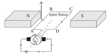
The force on side AB is vertically up (due to the right-hand palm rule).1 markThe force on side BC is zero since the current in BC and the magnetic field directions<br/>are parallel.1 mark
