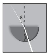
The data obtained is shown in the table below. The angle  $\theta_1$  represents the angle of incidence at the flat side of the block. The angle  $\theta_2$  represents the angle of refraction as the light enters the block. The light does not refract again as it leaves the curved side of the block.
