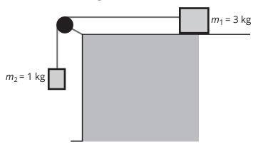
The string passes over a frictionless pulley and the mass of the string can be considered negligible.
