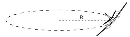
**b** The diagram below shows the only two unbalanced forces acting on the aircraft during the manoeuvre to fly the horizontal circle shown in part **a** of this question. Calculate the magnitude of the lift force,  $F_1$ . (3 marks)
