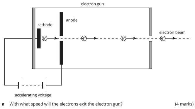
The electron gun's accelerating voltage was adjusted so that the exiting electrons were travelling at a speed of  $1.5 \times 10^5$  m s<sup>-1</sup>. The path taken by the electrons as they entered a magnetic field of strength 20 mT is shown below.
