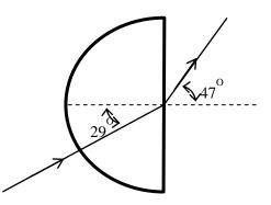
**a.** Determine the refractive index for the semicircular prism shown above. 2 marks
