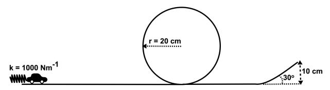
The spring constant for the launching spring is  $1000 \text{ Nm}^{-1}$ , the vertical loop has a radius of 20cm, and the jump is on an angle of  $30^{\circ}$ , with a height of 10 cm. The toy car has a mass of 50 grams.
