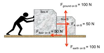
**c.**  $F_{of A on B} = 50 \text{ N}$  to the left (so that horizontal forces are balanced) According to Newton III,  $F_{Box A on Box B} = -F_{Box B on Box A}$ .
