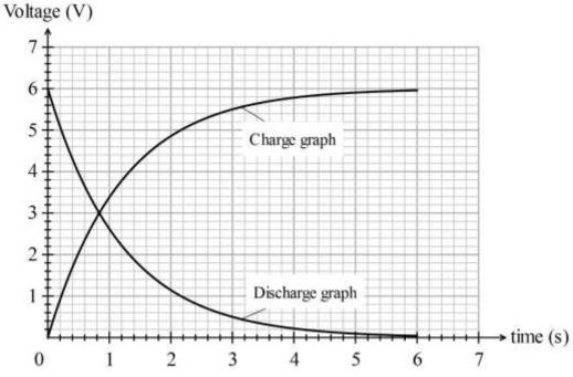
c. After 1.2 s, the capacitor is 63% charged 63% of voltage across the capacitor = 3.78V Voltage across R = 6 - 3.78 = 2.22 V
