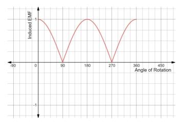
**c.** The split-ring commutator swaps the connection between the coil and the output every 1/2 turn. It swaps at the maximum flux position. This allows the current to keep flowing out of the generator in the same direction – DC.
