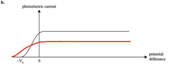
Horizontal intercept must be to the left of the original graph (due to higher cut-off potential caused by shorter wavelength/higher frequency light). Saturation current must be less than the original graph (due to reduced intensity).
