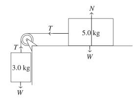
4 marks 1 mark for showing  $F_W$  for both masses. 1 mark for showing  $F_N$  on the 5.0 kg mass. 1 mark for showing  $F_T$  on the 5.0 kg mass with the correct direction. 1 mark for showing  $F_T$  on the 3.0 kg mass with the correct direction.
