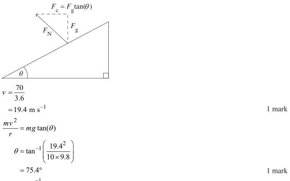
At 70 km  $h^{-1}$ , a banking angle of 75.4° is required to prevent the cyclist from coming off the banked section of the track. This is greater than the existing bank of the track.
