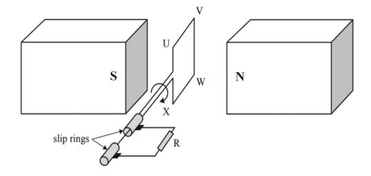
When the coil is rotating steadily, it takes 50 ms for each complete rotation and produces a peak EMF of 3.2 V.
