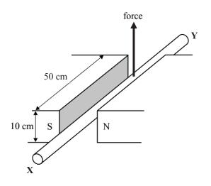
**a.** In which direction, X to Y or Y to X, is the current flowing in the rod?
