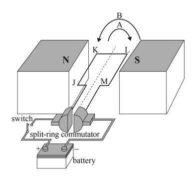
**a.** The current is switched on when the coil is stationary in the position shown in the diagram. The coil begins to rotate. Which of the directions of rotation (A or B) will the coil initially move?
