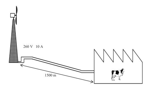
**a.** What RMS power is being produced by the wind generator?
