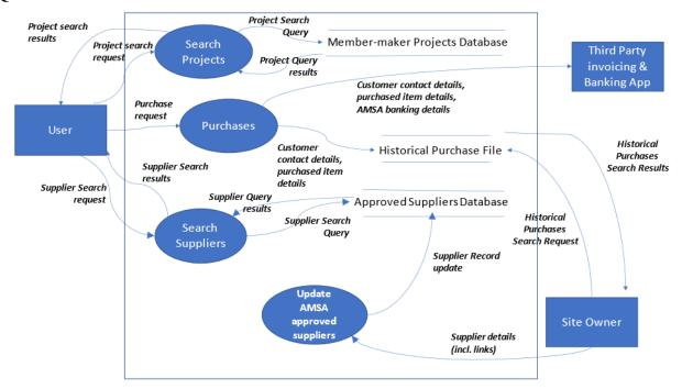
The Data Flow Diagram above shows the main processes for the new functions on the AMSA website.
