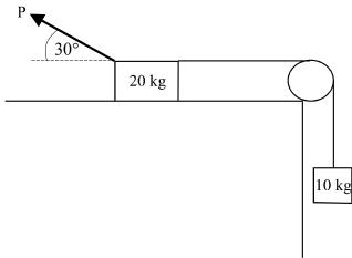
The normal force acting on the 20kg mass is *N* newton and the frictional force is *Fr* newton. In the diagram, the 20kg mass accelerates towards the left at  $a \text{ m/s}^2$ . For this system, which one of the following equations is true?
