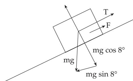
$$\begin{aligned}F + T - mg \sin 8^\circ &= 0 \\ T &= mg \sin 8^\circ - F \\ &= 1200 \times 9.8 \sin 8^\circ - F \\ &= 1636.68 - F\end{aligned}$$
