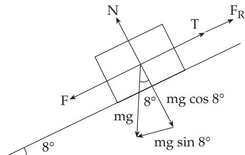
$$\begin{aligned}\text{Resultant force: } F_R &= ma \\ &= 1200 \times 0.25 \\ &= 300\end{aligned}$$
