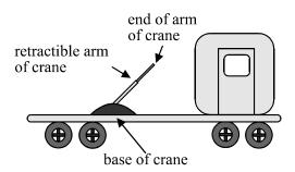
The arm of the crane can be rotated in such a way that the points in space that can be reached by the end of the arm of the crane form a solid in the shape of an inverted cone with a curved top, as shown in the diagram below.
