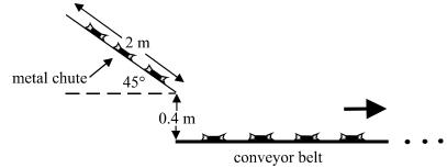
The coefficient of friction between a lolly and the metal chute is 0.5. The forces acting on a lolly, (each of which have a mass of 0.025kg) as it slides down the metal chute are the weight force, the normal reaction and the friction force.
