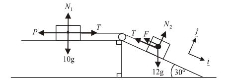
$N_1$  and  $N_2$  are the normal forces acting on the 10kg and 12kg masses respectively. *F* is the friction force of the inclined plane on the 12kg mass.
