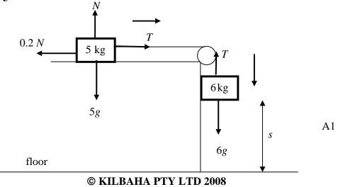
let a be the acceleration of the system, and T the tension in the string. resolving horizontally on the table around the 5 kg block.
