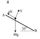
From the diagram:  $40g \sin 35^\circ - \mu N = 40 \times \frac{9}{10}$  and  $N - 40g \cos 35^\circ = 0$ . It follows  $40g \sin 35^\circ - \mu \times 40g \cos 35^\circ = 40 \times \frac{9}{10}$  M1  $\mu = \frac{g \sin 35^\circ - 0.9}{g \cos 35^\circ} = 0.575$  A1
