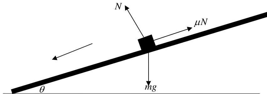
resolving perpendicular to the plank
