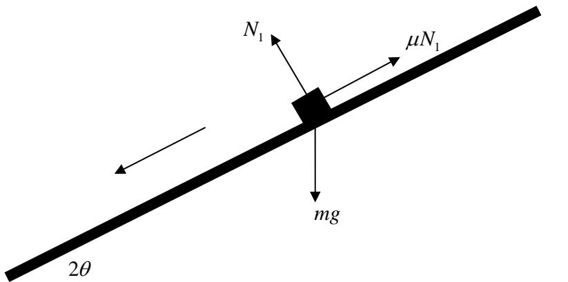
resolving perpendicular to the plank
