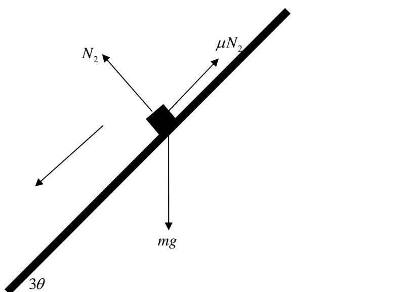
resolving perpendicular to the plank
