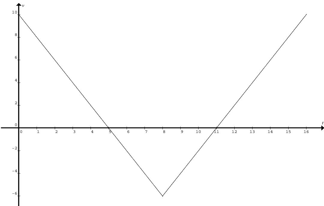
The distance from the start, is the signed area of the triangles, or displacement
