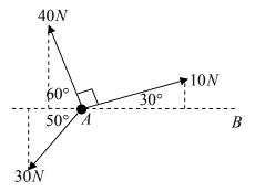
Sum of perpendicular components =  $40 \sin 60^\circ - 30 \sin 50^\circ + 10 \sin 30^\circ = 16.66$  (2 dec.pl).
