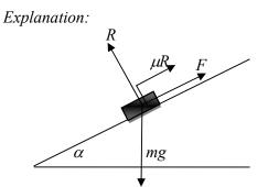
Resolving horizontally:  $F + \mu R - mg \sin \alpha = 0$ Resolving vertically:  $R - mg \cos \alpha = 0 \Rightarrow R = mg \cos \alpha$ Therefore,  $F = mg \sin \alpha - \mu mg \cos \alpha = mg(\sin \alpha - \mu \cos \alpha)$ .
